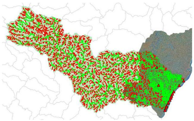
Figure A2.13 Snapshot of the SWMM model of the Southern EMA catchments.
