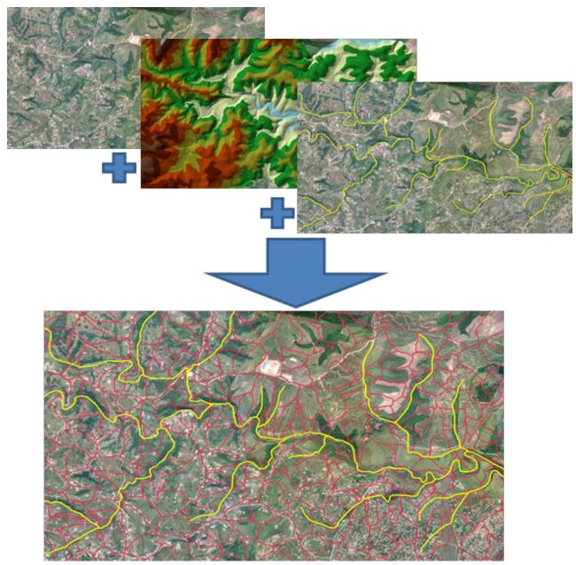
Figure A2.2 Information required to delineate subcatchments: topographical aerial survey, DEM and river centre lines based on river flow paths
