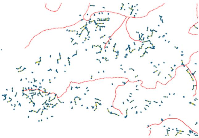
Figure A2.5 Current available stormwater shapefile (the red lines represent the flow paths, yellow lines are stormwater conduits and blue dots represent stormwater junctions).
