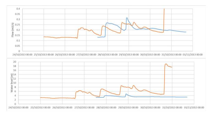
Figure A2.16 Measured (gauge U2H022, orange line) vs simulated flows (blue line) and water levels on the Msunduze (Umgeni) River.
