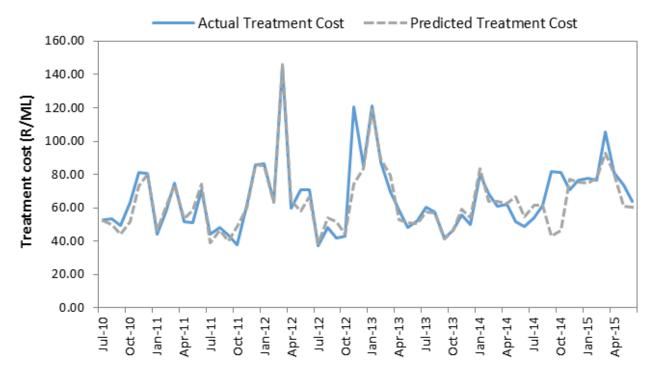
Figure A5.4 Actual versus predicted water treatment costs fitted using the treatment cost model estimates for Durban Heights WTW
