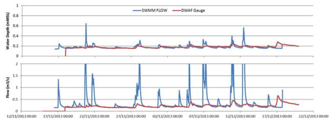
Figure A2.18 Measured (red line) vs simulated flows (blue line) and water levels on the Nungwane River in the south.
