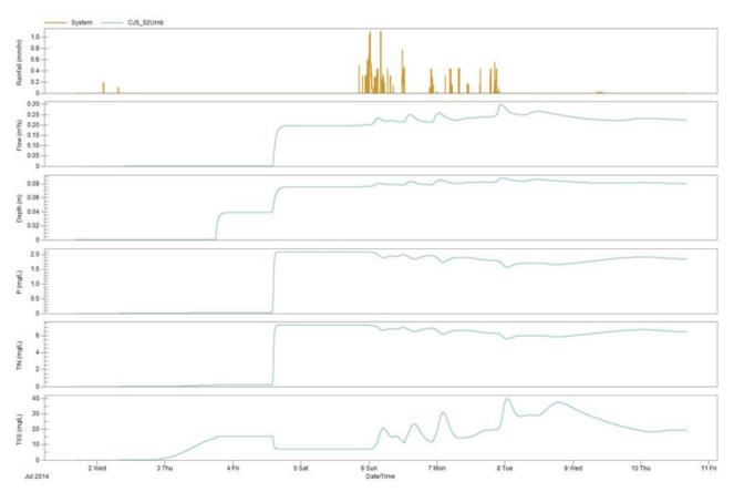
Figure A2.20 Measure rainfall and simulated flow, depth, P, TIN, TSS concentrations for monitoring station (R\_ZANA\_10) on the Umhlatuzana River.
