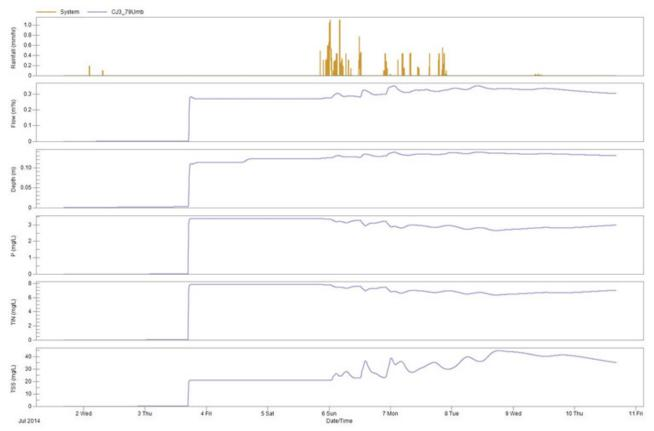
Figure A2.21 Measure rainfall and simulated flow, depth, P, TIN, TSS concentrations for monitoring station (R\_UMBILO\_13) on the Umbilo River.
