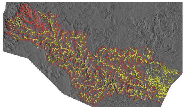
Figure A2.19 The southern EThekwini catchments showing the additional conduits that were included in the model represented by the red lines.
