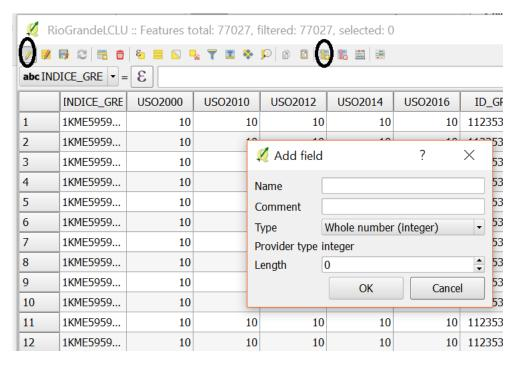
2) Name the field: AREA\_SQKM. Change type to Float and length to 50. Calculate area.
