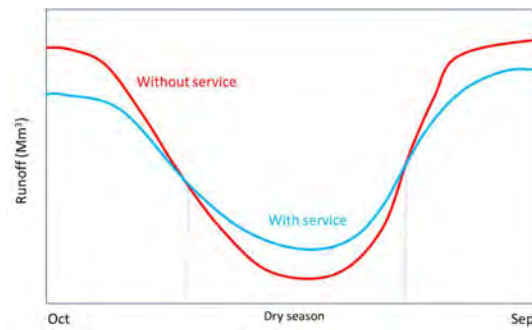
Figure 4.17. Schematic diagram of the effects of infiltration and temporary storage by river basin ecosystems on the seasonal patterns of surface water flow from the river basin.
