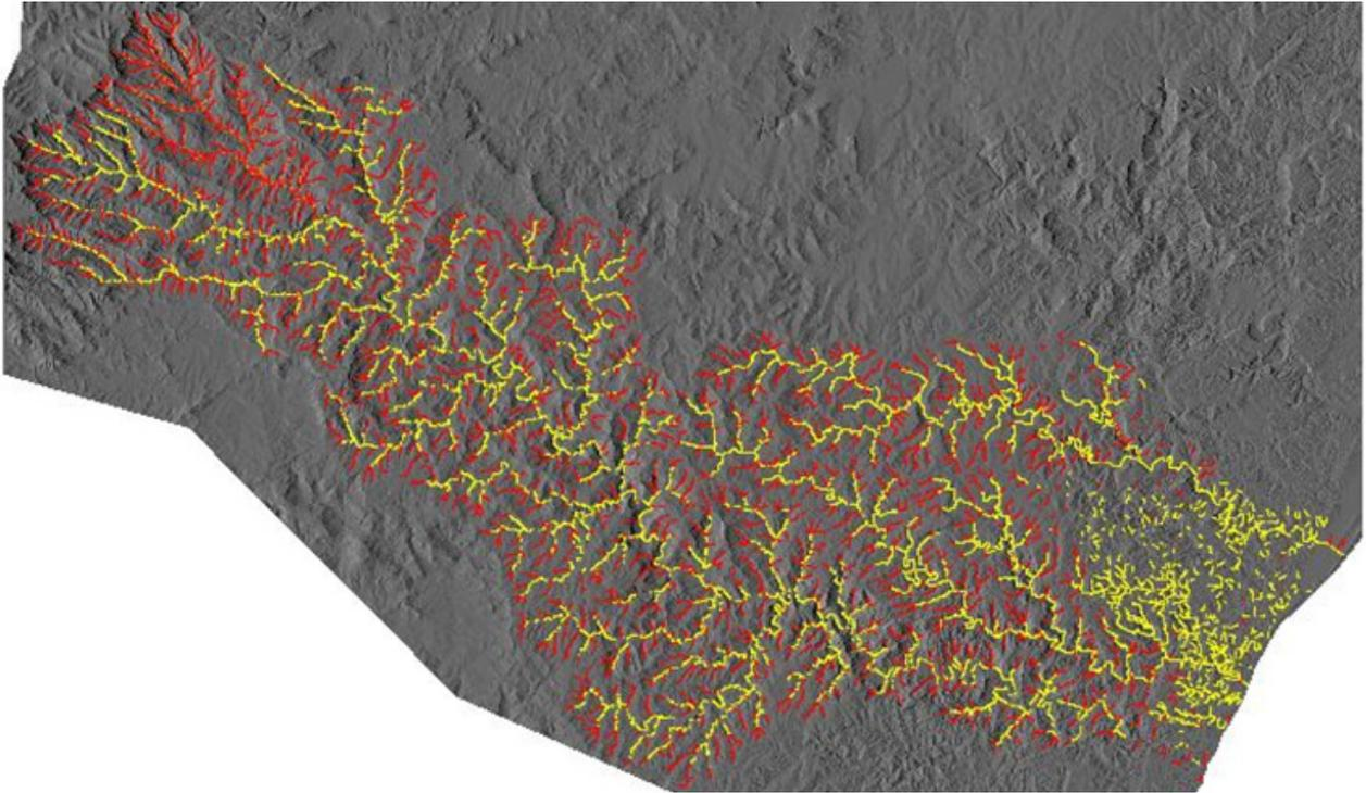
**Figure A2.19** The southern EThekweni catchments showing the additional conduits that were included in the model represented by the red lines.
