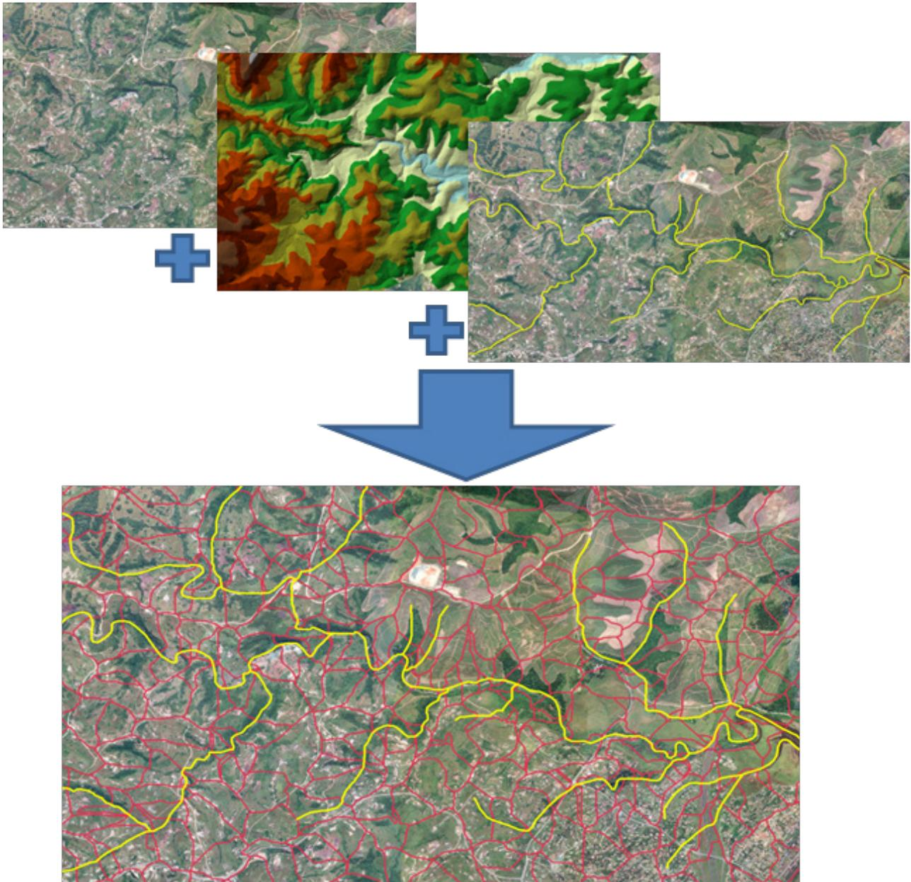
**Figure A2.2** Information required to delineate subcatchments: topographical aerial survey, DEM and river centre lines based on river flow paths
