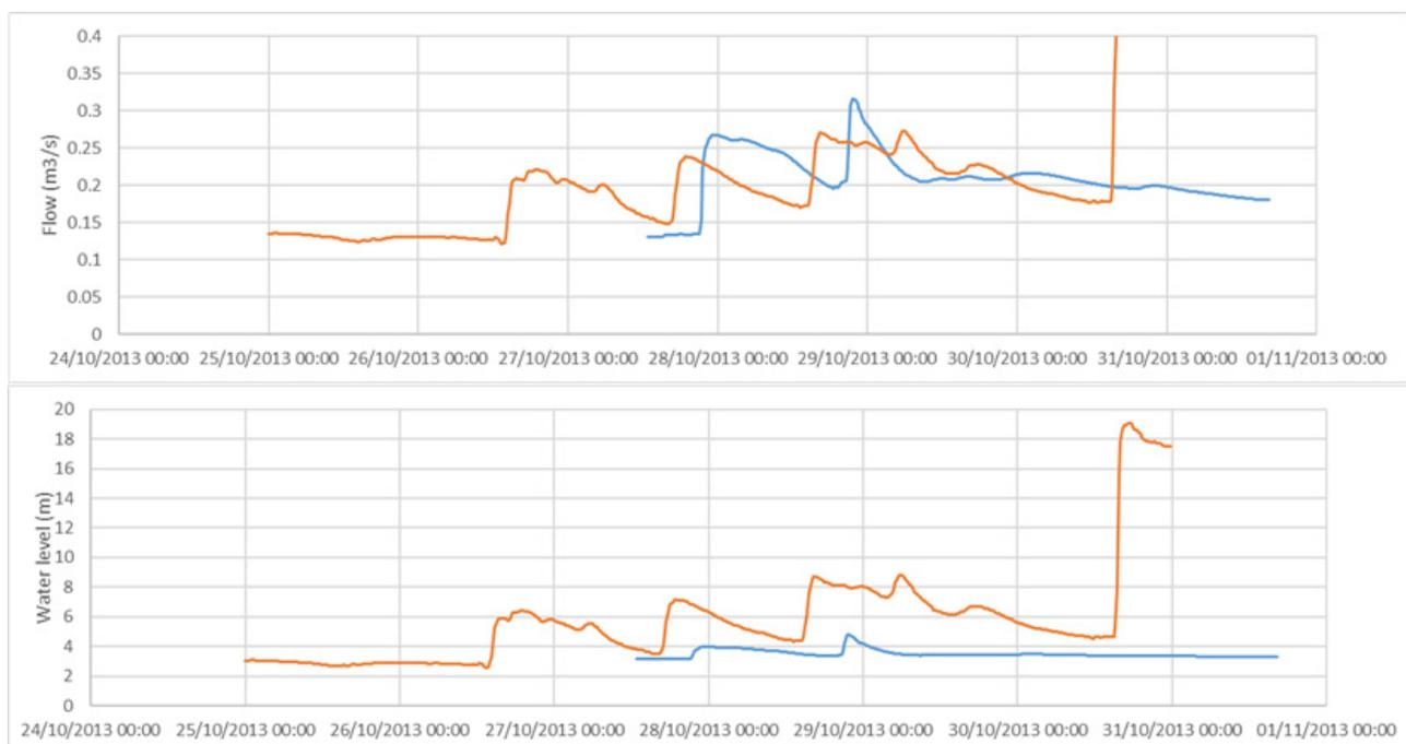
Figure A2.16 Measured (gauge U2H022, orange line) vs simulated flows (blue line) and water levels on the Msunduze (Umgeni) River.
