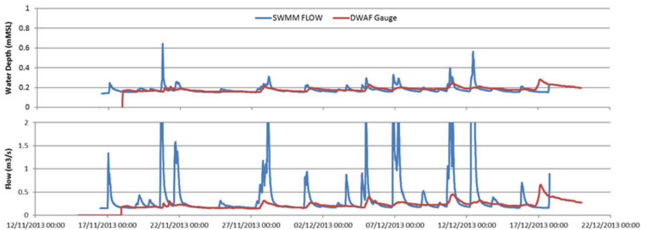
Figure A2.18 Measured (red line) vs simulated flows (blue line) and water levels on the Nungwane River in the south.
