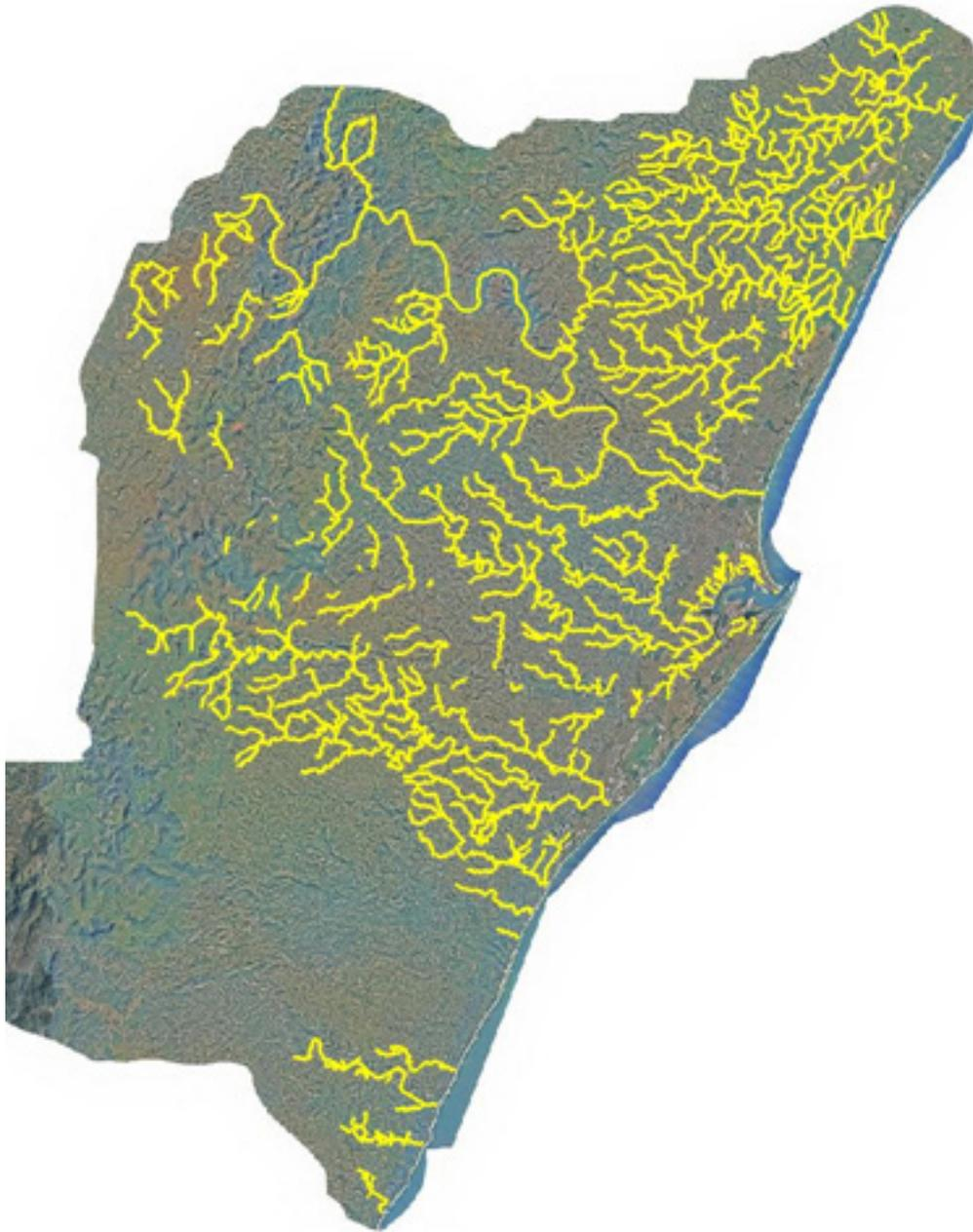
**Figure A2.3** Illustration of HecRAS files merged and converted to SWMM5 layers for the study
