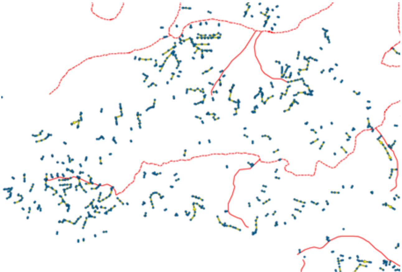
**Figure A2.5** Current available stormwater shapefile (the red lines represent the flow paths, yellow lines are stormwater conduits and blue dots represent stormwater junctions).
